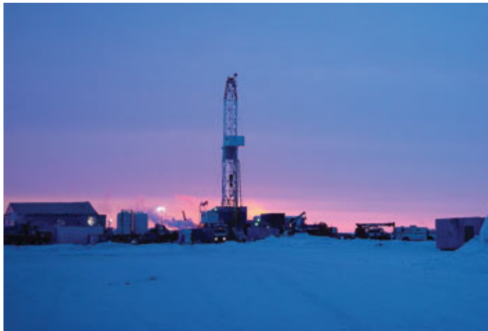
An international team of researchers at the Mallik site in the Northwest Territories drilled three 3,900-foot wells during the winter of 2002. They found that gas production from hydrate was technologically feasible.
